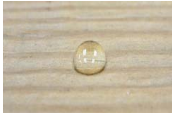
Encore™ NF55E with 9 months horizontal exposure
