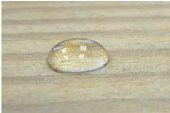
Commercially available stain with 9 months horizontal exposure
